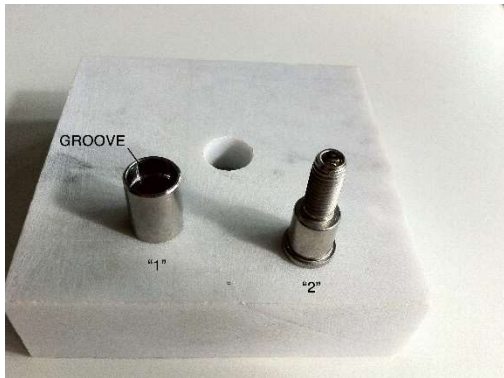
Anchor components: 1: Sleeve, 2: Threaded pin Behind the components, the undercut hole
