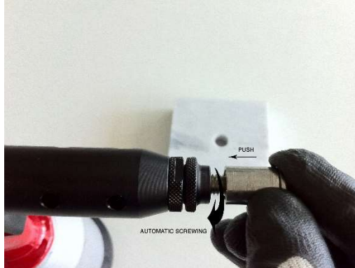
Anchor screwing on to the pneumatic tool: push it against the tool hub to activate the automatic screwing
