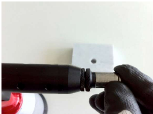
End of screwing on the pneumatic tool. The sleeve edge is in contact with the tool
