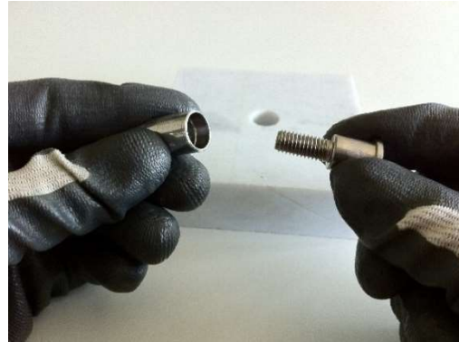
Anchor component joining: join the sleeve to the pin from the groove side
