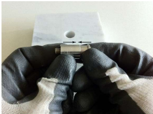
Anchor component joining: push the sleeve to the end of the pin
