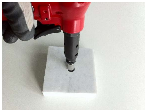
Anchor inserting into the undercut hole
